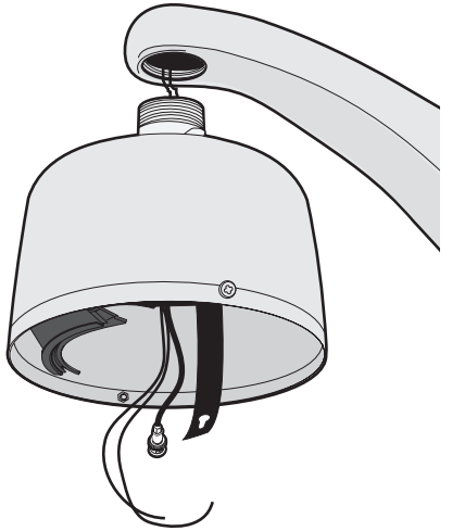
Figure 6. Attaching the Pendant Back Box to the Mount
