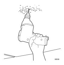
a. Locate the center point of the mounting location. Drill a hole in the ceiling using a 3/32-inch drill.
