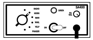
The **OFF/ON** Toggle Power Switch controls the siren power. The power should be turned off when not being used to conserve battery power.
