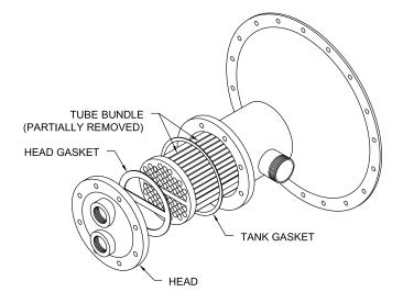
4. When replacing the heat exchanger head, use a torque wrench to tighten the bolts/studs and nuts. Use the following chart as a guide. All torque values apply to well-lubricated nut bearing surfaces.
