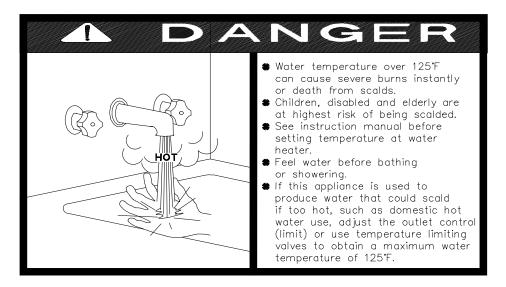
Thermostatically controlled mixing values must be used in the design of the potable hot water system.
