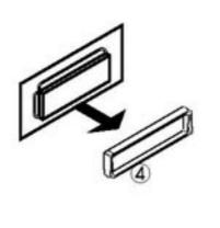
Insert the keys supplied with the unit at both sides of the unit as shown in figure until they click. Pulling the keys makes it possible to remove the unit from the dashboard.
