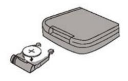
Insert the Battery Holder into the Remote Control.
