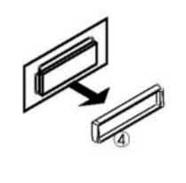
Insert the keys supplied with the unit at both sides of the unit as shown in figure until they click. Pulling the keys makes it possible to remove the unit from the dashboard.
