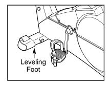
slightly during use, turn one or both of the leveling feet under the front stabiliser until the rocking motion is eliminated.
