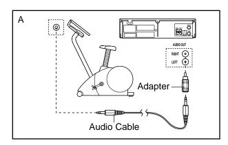
B. Plug one end of the audio cable into the jack beneath the console of the exercise cycle. Plug the other end of the cable into the included adapter. Plug the adapter into an RCA adapter (available at electronics stores). Next, remove the wire that is currently plugged into the AUDIO OUT jack on your VCR and plug the wire into the unused side of the RCA adapter. Plug the RCA adapter into the AUDIO OUT jack on your VCR.
