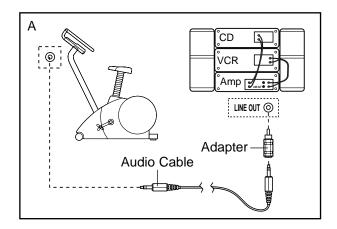
B. Plug one end of the audio cable into the jack beneath the console of the exercise cycle. Plug the other end of the cable into the included adapter. Plug the adapter into an RCA Y-adapter (available at electronics stores). Next, remove the wire that is currently plugged into the LINE OUT jack on your stereo and plug the wire into the unused side of the RCA Y-adapter. Plug the RCA Y-adapter into the LINE OUT jack on your stereo.
