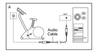
B. Plug one end of the audio cable into the jack beneath the console of the exercise cycle. Plug the other end of the cable into a 3.5mm Y-adapter (available at electronics stores). Plug the Y-adapter into the PHONES jack on your computer. Plug your headphones or speakers into the other side of the Y-adapter.
