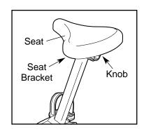
may scratch the seat bracket). Next, pull the knob, slide the seat to the desired position, and then release the knob. Move the seat bracket forward and backward slightly until the pin on the knob snaps into one of the holes in the seat bracket. Then, turn the knob clockwise until it is tight.
