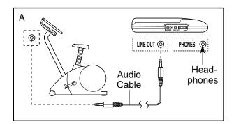
B. Plug one end of the audio cable into the jack beneath the console of the exercise cycle. Plug the other end of the cable into a 3.5mm Y-adapter (available at electronics stores). Plug the Y-adapter into the PHONES jack on your CD player. Plug your headphones into the other side of the Yadapter.
