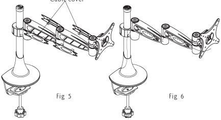
Route the cables along one side of the Inner Arm (nearest the wall plate). With cables in place, loosely secure the Inner Arm cable covers back in place. Next, route the cables along the opposite side of the Outer Arm. Be sure to leave slack in the cable where it transitions between two sides of the Arm Assembly. With cables in position, loosely secure the Outer Arm cable covers back in place.
