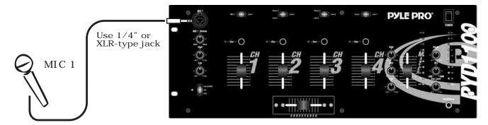
Microphone 2. Connect a high quality balanced/unbalanced low impedance (600 Ohm) microphone with a 1/4" plug to the MIC  $\tilde{z}$  jack on the lower left corner of the mixer's back panel.
