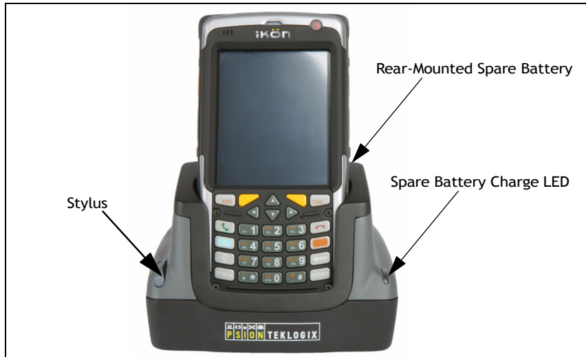
Figure 7.3 CH4000 Desktop Docking Station - Front View
