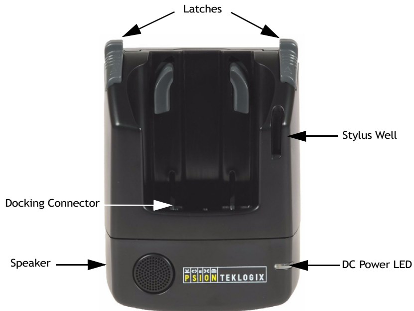
Figure 6.12 CH1005A Front View
