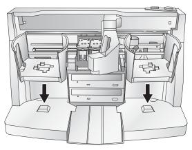
• Load the Input Bin (the bin located on the right-hand side of the Publisher) with 50 blank discs and place the bins on the mounting pegs.
