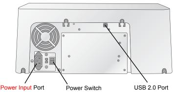
The **USB 2.0 Port** is connected to an open USB 2.0 port on your PC with the USB 2.0 cable, included with your Publisher.
