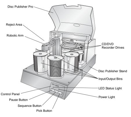
The **Robotic Arm** transports discs from an Input Bin, to a CD/DVD Recorder, to the printer, and finally to an Output Bin.
