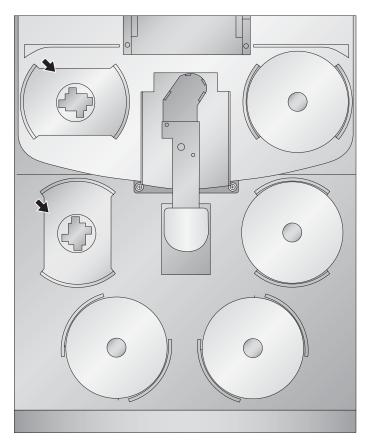
• Load up to 50 discs into the right bin of the Disc Publisher Pro and up to 25 discs in a Disc Publisher.
