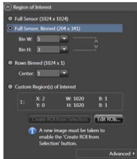
Figure 5-17: Dual Port Readout: LightField Settings, 5x3 Binning, Interline CCD
