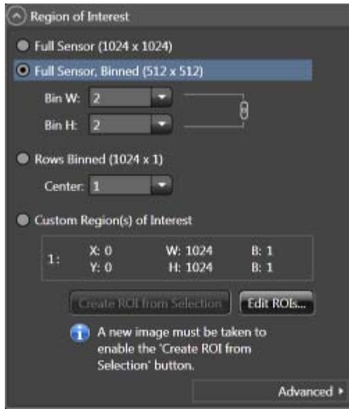
Figure 5-12: Dual Port Readout: LightField Setting, 2x2 Binning, Interline CCD
