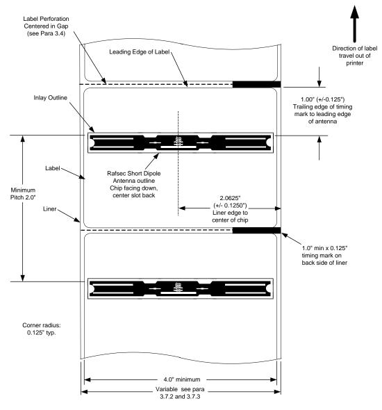
Printronix RFID Label Requirements for Rafsec Short Dipole Inlay
