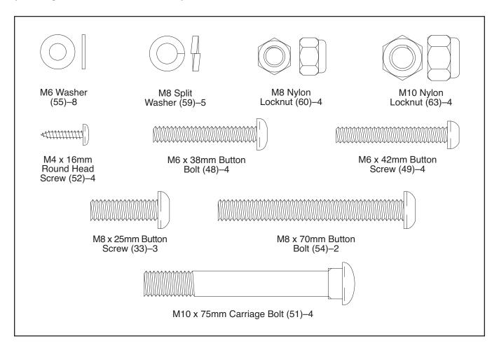
While another person lifts the front of the Frame (1) slightly, attach the Front Stabilizer (3) to the Frame with two M10 x 75mm Carriage Bolts (51) and two M10 Nylon Locknuts (63).
