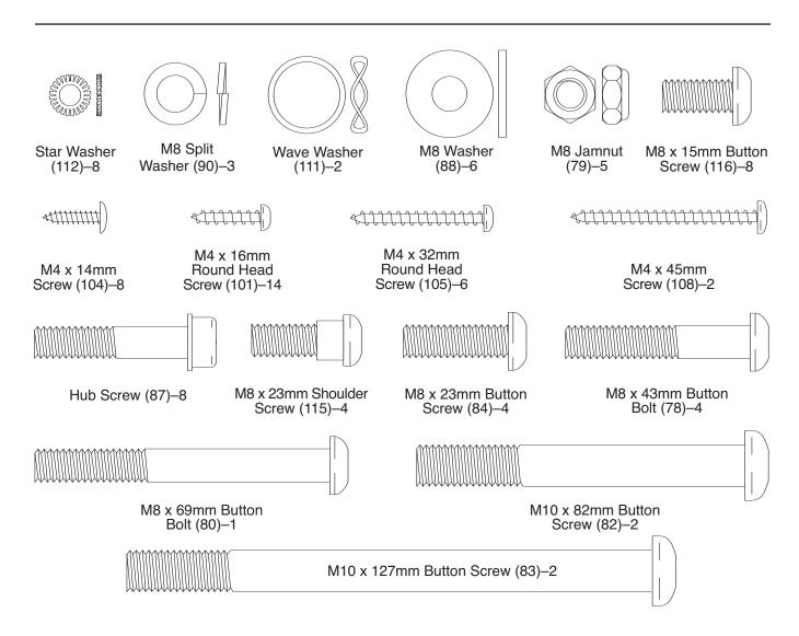
1. While another person lifts the Base (1), attach the Front Stabilizer (6) to the Base with two M10 x 82mm Button Screws (82).
