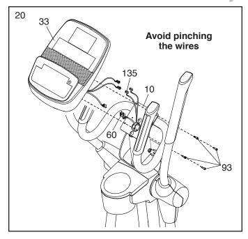
21. Attach the Console Cover (11) to the Console (33) with two M4 x 16mm Screws (93).
