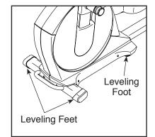
If the frame of the elliptical flexes
