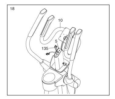
19. Insert the Upright Wire (60) and the Pulse Wires (135) upward through the Handlebar (10).
