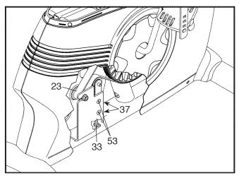
Then, reattach the right shield, the top shield, and the top shield cap. Reattach the right pedal, if necessary.
