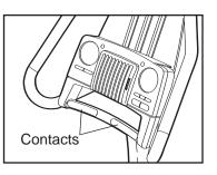
the handgrip pulse sensor, with your palms on the contacts closest to you and your fingers touching the contacts on the opposite side of the handgrip pulse sensor. **Avoid moving your hands.** When your pulse is detected, the heart-shaped indicator in the upper part of the display will begin to flash each time your heart beats. After a moment your heart rate will be shown.
