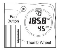
If the fan is turned on but the pedals are not moved for thirty seconds, the fan will automatically turn off.
