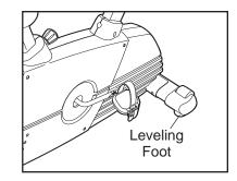
ly during use, turn one or both of the leveling feet under the front stabilizer until the rocking motion is eliminated.
