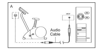
B. Plug one end of a 1/8" to 1/8" stereo audio cable (available at electronics stores) into the jack beneath the console. Plug the other end of the cable into a 1/8" Y-adapter (available at electronics stores). Plug the Y-adapter into the PHONES jack on your computer. Plug your headphones or speakers into the other side of the Y-adapter.
