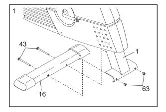
Orient the Front Stabilizer (15) as shown. Attach the Front Stabilizer to the Frame (1) with two M10 x 112mm Carriage Bolts (43) and two M10 Nylon Locknuts (63).
