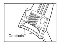
the handgrip pulse sensor, with your palms on the contacts closest to you and your fingers touching the contacts on the opposite side of the handgrip pulse sensor. **Avoid moving your hands.** When your pulse is detected, the heart-shaped indicator in the upper part of the display will begin to flash each time your heart beats. After a moment, the display will show your heart rate.
