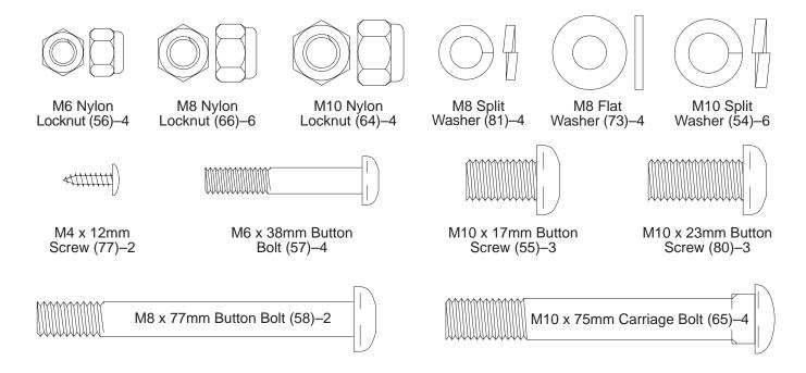
1. Attach one of the Stabilizers (19) to the front of the Frame (1) with two M10 x 75mm Carriage Bolts (65) and two M10 Nylon Locknuts (64).
