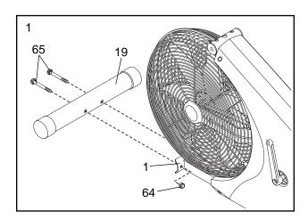
2. Attach the other Stabilizer (19) to the rear of the Frame (1) with two M10 x 75mm Carriage Bolts (65) and two M10 Nylon Locknuts (64).
