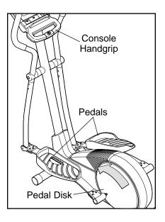
ommended that you move the pedal disks in the direction shown by the arrow; however, for variety, you may turn the pedal disks in the opposite direction.
