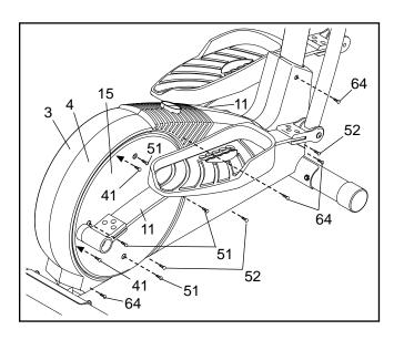
Next, remove the four Screws (51) from the right Pedal Disc (15), and slide the Pedal Disc off. Remove all Screws (52, 64) from the Right Side Shield (4) and the two Bolts (41) from beneath the Pedal Disc, and remove the Right Side Shield (4). Remove all Screws (52) from the Left Side Shield (3), and remove the Left Side Shield.
