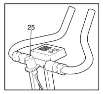
resistance, turn the Resistance Knob clockwise; to decrease the resistance, turn the Resistance Knob counterclockwise.
