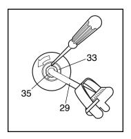
(33). Lightly tap the screwdriver with a hammer to turn the Slotted Bearing Nut counterclockwise until the arms are no longer loose. **Do not overtighten the Slotted Bearing Nut.** When the Slotted Bearing Nut is properly tightened, tighten the Crank Nut.
