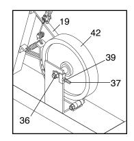
tighten the M8 Flanged Hex Nuts (36). Reattach the side shields.
