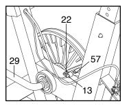
the Screw. Turn the Crank (29) for a moment. Repeat until the console displays correct feedback. When the Reed Switch is correctly adjusted, reattach the left side shield.
