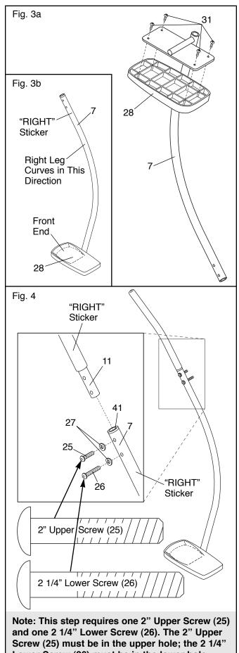
Lower Screw (26) must be in the lower hole.
