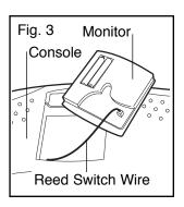
If the electronic monitor still does not function properly, the batteries should be replaced. Two "AA" batteries are required; alkaline batteries are recommended. Remove the two old batteries from the monitor, and insert two new batteries. Make sure that the negative (–) ends of the batteries are touching the springs, and that the positive (+) ends of the batteries are pushed against the metal contacts.
