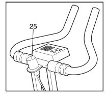
the Resistance Knob clockwise; to decrease the resistance, turn the Resistance Knob counterclockwise.
