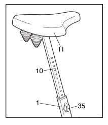
remove the Seat Pin (35). Align one of the holes in the Seat Post (10) with the hole in the Frame (1). Insert the Seat Pin into the Frame and the Seat Post. Caution: Make sure to insert the Seat Pin through one of the holes in the Seat Post; do not insert the Seat Pin under the Seat Post.
