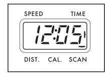
a flashing mode indicator will show which mode is currently displayed. Note: If a different mode is selected, you can select the scan mode again by repeatedly pressing the mode button. Speed, time, distance or calorie mode—
