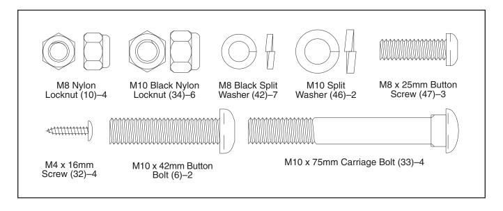
1. Identify the Front Stabilizer (2). While another person lifts the front of the Frame (1) slightly, attach the Front Stabilizer to the Frame with two M10 x 75mm Carriage Bolts (33) and two M10 Black Nylon Locknuts (34).
