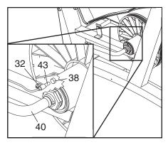
indicated M4 x 16mm Screw (32). Slide the Reed Switch slightly closer to or away from the Magnet, and then retighten the Screw. Turn the Crank Arm for a moment. Repeat until the console displays correct feedback. When the Reed Switch is correctly adjusted, reattach the left side shield, the side shield cover, and the left pedal.
