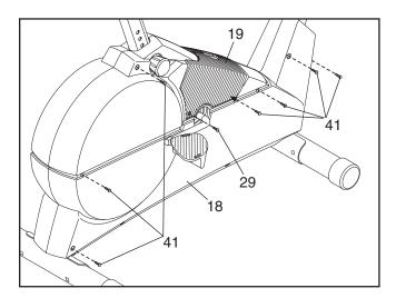
Using an adjustable wrench, turn the Left Pedal (24) clockwise and remove it. Next, remove the two M4 x 16mm Screws (32) from the Left Side Shield (17) and the M4 x 12mm Round Head Screw (29) from the Side Shield Cover (19). Lift off the Side Shield Cover and the Left Side Shield.
