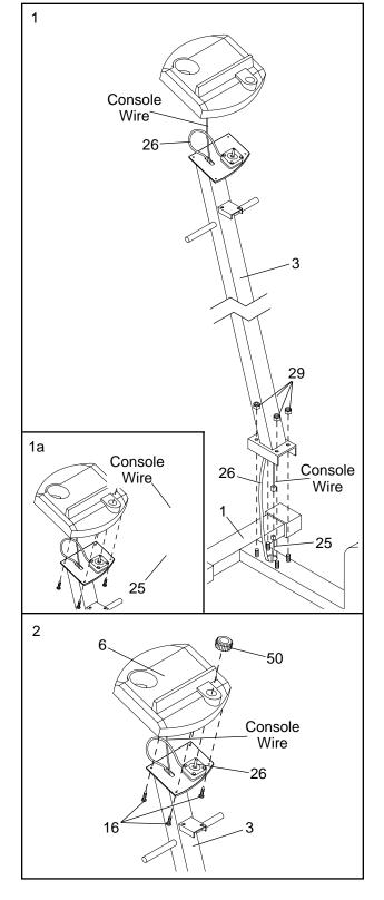
Feed the console wire back down into the Upright (3). Attach the Console (6) to the Upright with four #8 x 3/4" Round Head Screws (16). Be careful to avoid pinching the console wire.
