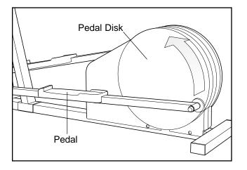
To dismount the 485E, allow the pedals to come to a complete stop. **CAUTION: The 485E does not have a freewheel; the pedals will continue to move until the flywheel stops.** When the pedals are stationary, step off the highest pedal first. Then, step off the lowest pedal.
