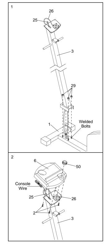
While another person holds the Console (6) near the Upright (3), connect the console wire to the Sensor Wire (25).
