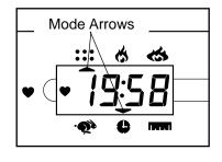
flashing mode arrow will show which mode is currently displayed. Note: If a different mode is selected, you can select the scan mode again by repeatedly pressing the mode button.
