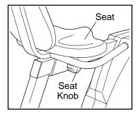
the seat knob counterclockwise to loosen it (if the seat knob is not loosened enough, it may scratch the frame). Next, slide the seat to the desired position, and then retighten the seat knob. **IMPORTANT:** After you adjust the seat, make sure that your knees will not touch the handlebar or the console when you pedal.
