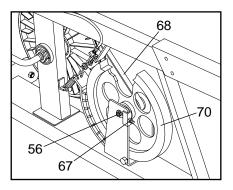
If the Belt is properly adjusted, reattach the side shields and pedals. If the Belt needs to be adjusted, loosen the M8 Nylon Locknut (56) on each side of the Flywheel (70). To tighten the Belt, turn the two Adjustment Nuts (67) clockwise; to loosen the Belt, turn the Nuts counterclockwise. Make sure that the Flywheel is straight and tighten the M8 Nylon Locknuts (56). Reattach the side shields and pedals.
