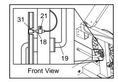
remove the M4 x 16mm Screw (21). Slide the Reed Switch slightly closer to or away from the Magnet. Retighten the Screw. Turn the Crank for a moment. Repeat until the console displays correct feedback. When the Reed Switch is correctly adjusted, reattach the left side shield and the pedal.
