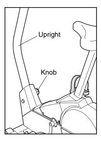
the knob. Move the upright up and down slightly until the pin on the knob snaps into one of the holes in the upright. Then, turn the knob clockwise until it is tight.
