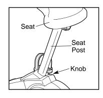
indicated knob counterclockwise two or three turns to loosen it (if the knob is not loosened enough, it may scratch the seat post). Next, pull the knob, slide the seat post to the desired height, and then release the knob. Move the seat post up and down slightly until the pin on the knob snaps into one of the holes in the seat post. Then, turn the knob clockwise until it is tight.
