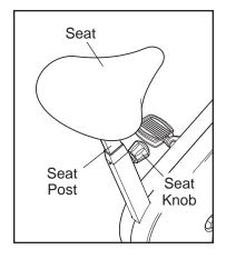
knob, raise or lower the seat post, and then release the seat knob. Move the seat post up and down slightly until it locks into position. Then, tighten the seat knob. CAUTION: Make sure that the pin on the seat knob is inserted into one of the adjustment holes in the seat post. Do not rest the seat post on top of the pin on the seat knob.
