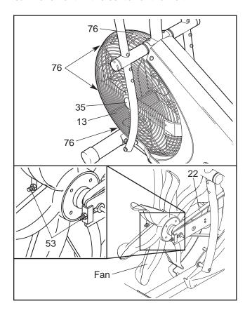
If the Belt (22) needs to be adjusted, loosen the right Guard Fastener (not shown). To tighten the Belt, turn the M6 Nuts (53) clockwise; to loosen the Belt, turn the M6 Nuts counterclockwise. Make sure that the fan is straight, and then reattach the Left Guard, tighten the Guard Fasteners, and reattach the Guard Clips.
