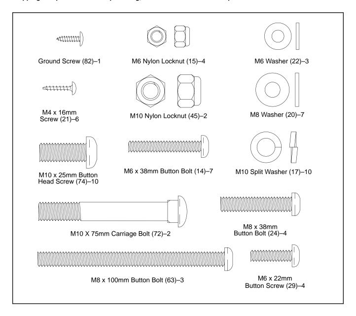
Attach the Front Stabilizer (2) to the front of the Frame (1) with two M10 x 75mm Carriage Bolts (72) and two M10 Nylon Locknuts (45). Make sure that the Front Stabilizer is turned so the Wheels (75) are not touching the floor.
