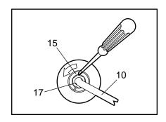
screwdriver with a hammer to turn the Slotted Crank Nut counterclockwise until the arms are no longer loose. **Do not overtighten the Slotted Crank Nut.** When the Slotted Crank Nut is properly tightened, retighten the Crank Nut and re-attach the left side shield.
