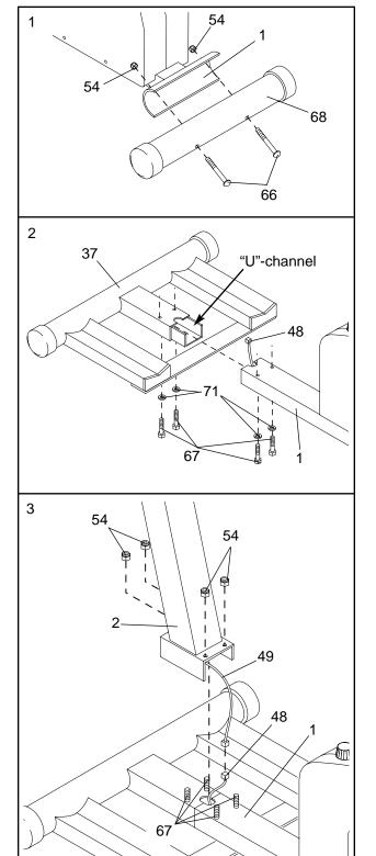
Slide the "U"-channel on the Rail Stabilizer (37) into the Base (1). Make sure that the Reed Switch Wire (48) is extending from the hole formed where the two parts meet; be careful not to damage the Reed Switch Wire.
