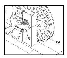
removed for clarity). Slide the Reed Switch slightly toward or away from the Magnet. Make sure that the Magnet will not hit the Reed Switch. Retighten the Screw. Turn the Pulley (19) for a moment. Repeat until the console displays correct feedback. When the Reed Switch is correctly adjusted, re-attach the left side shield.
