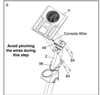
7. Slide the Console Cover (96) (see the drawing in step 6) upward to the Console (4). Attach the Console Cover with four M4 x 16mm Round Head Screws (94).
