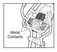
handgrips with your palms resting against the metal contacts. Avoid moving your hands or squeezing the handgrips too tightly; excessive movement or pressure may interfere with heart rate readings. When your pulse is detected, the heart-shaped indicator in the large display will flash each time your heart beats, and your heart rate will be shown.
