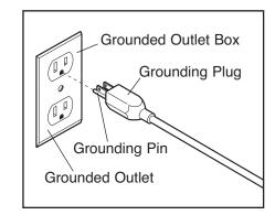
reduce the risk of electric shock. This product is equipped with a cord having an equipment-grounding conductor and a grounding plug. Plug the power cord into an appropriate outlet that is properly installed and grounded in accordance with all local codes and ordinances. This product is for use on a nominal 120-volt circuit. Important: The elliptical exerciser is not compatible with GFCI-equipped outlets.
