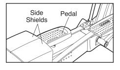
step onto the other pedal. Push the pedals until they begin to move with a continuous motion. Note: The crank arms (inside of the side shields) can be turned in either direction. It is recommended that you turn the crank arms in the same direction that you pedal a bicycle; however, for variety, you can turn the crank arms in the opposite direction.
