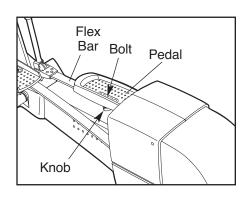
the pedal. Next, push the bolt upward, slide the pedal forward or backward to the desired position, and then retighten the knob. Make sure that both pedals are in the same position.
