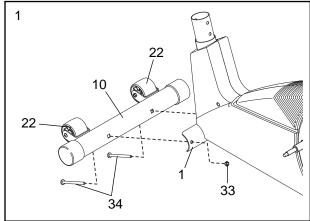
While another person lifts the back of the Frame (1), attach the Rear Stabilizer (9) to the Frame with two M10 x 75mm Carriage Bolts (34) and two M10 Nylon Locknuts (33).
