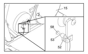
When the Reed Switch (53) is correctly adjusted, reattach the Side Shields (3, 4), the right Pedal Disc (15), the Pedal Arms (11, 12), and the Pedals (13, 14).
