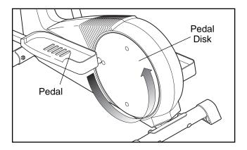
To dismount the elliptical trainer, allow the pedals to come to a complete stop. **CAUTION: The elliptical trainer does not have a free wheel; the pedals will continue to move until the flywheel stops.** When the pedals are stationary, step off the highest pedal first. Then, step off the lowest pedal.
