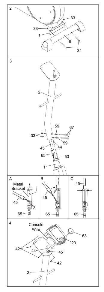
3. While another person holds the Upright (2) near the Frame (1) as shown, connect the Upper Wire (44) to the Reed Switch Wire (53).
