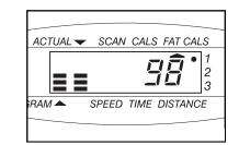
display, repeatedly press the display button until an arrow appears below or above the desired mode. Make sure that there is not an arrow under the word "scan."
