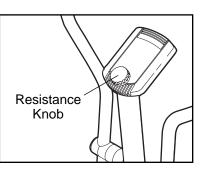
decrease the resistance, turn the knob counterclockwise. Important: The knob may not stop turning when maximum or minimum resistance is reached. When the knob becomes more difficult to turn, stop turning it or damage will result.
