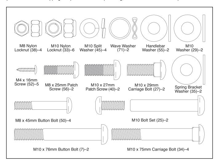
Identify the Front Stabilizer (10), which has round Endcaps (21). While another person lifts the front of the Frame (1), attach the Front Stabilizer to the Frame with two M10 x 75mm Carriage Bolts (34) and two M10 Nylon Locknuts (33).
