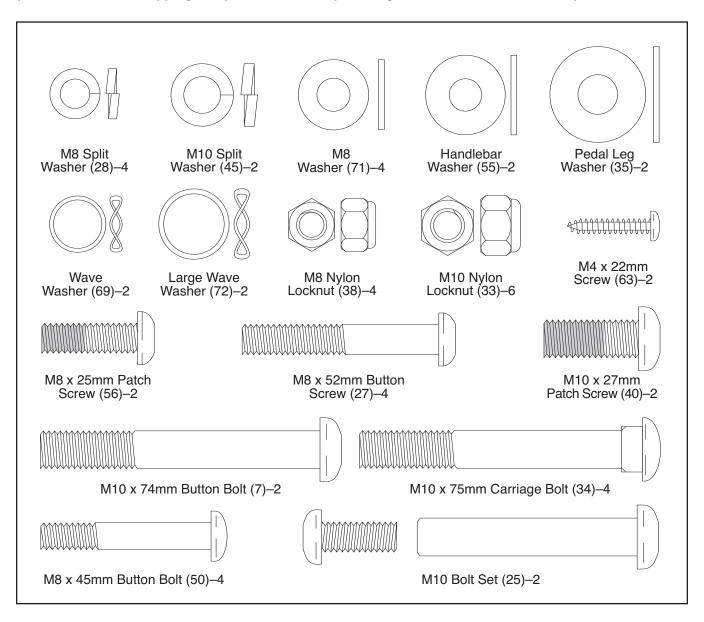
Identify the Front Stabilizer (10), which has round Endcaps (21) on its ends. While another person lifts the front of the Frame (1), attach the Front Stabilizer to the Frame with two M10 x 75mm Carriage Bolts (34) and two M10 Nylon Locknuts (33).
