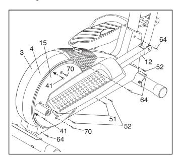
Next, remove the four Screws (51, 70) from the right Pedal Disc (15), and slide the Pedal Disc off. Remove all Screws (52, 64) from the Right Side Shield (4) and the two Bolts (41) from beneath the Pedal Disc, and remove the Right Side Shield (4). Remove all Screws (52) from the Left Side Shield (3), and move the Left Side Shield.
