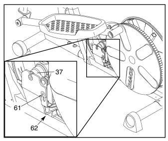
Next, loosen the M8 x 19mm Flat Head Bolt (61) and turn the Adjustment Screw (62) until the Belt (37) is tight. Once the Belt is tight, tighten the Flat Head Bolt. Then, reattach the side shields. Note: If you have questions regarding which screw should be in which hole, see EXPLODED DRAWING B on page 19 and the PART LIST on page 17.
