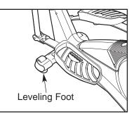
rocks slightly during use, turn one or both of the leveling feet under the front stabilizer until the rocking motion is eliminated.
