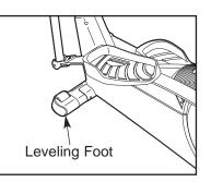
rocks slightly during use, turn one or both of the leveling feet under the front stabilizer until the rocking motion is eliminated.
