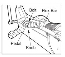
pedal forward or backward to the desired position, and then retighten the knob. Make sure that both pedals are in the same position.
