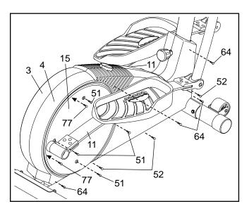
Next, remove the four Screws (51) from the right Pedal Disc (15), and slide the Pedal Disc off. Remove all Screws (52, 64) from the Right Side Shield (4) and the two Screws (77) from beneath the Pedal Disc, and remove the Right Side Shield (4). Remove all Screws (52) from the Left Side Shield (3) and remove the Left Side Shield.
