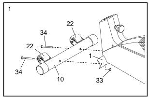
While another person lifts the back of the Frame (1), attach the Rear Stabilizer (9) to the Frame with two M10 x 75mm Carriage Bolts (34) and two M10 Nylon Locknuts (33).
