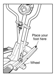
place one foot against the ramp and lower the elliptical crosstrainer. Due to the size and weight of the elliptical crosstrainer, use extreme caution while moving and lowering it.
