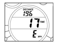
center of the large display will show the total number of hours that the elliptical crosstrainer has been used. The lower section of the large display will show an E for English miles or an M for metric kilometers. To change the unit of measurement, press the Resistance + button.
