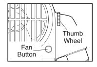
the fan, press the fan button a third time. Note: If the pedals are not moved for about thirty seconds, the fan will automatically turn off.
