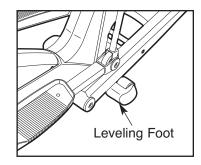
under the front stabilizer until the rocking motion is eliminated.
