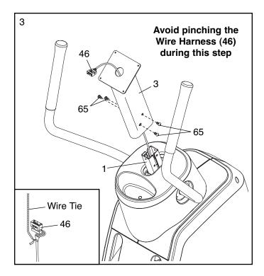
While a second person holds the Console (4) near the Upright (3), connect the console wire to the Wire Harness (46). Insert the excess wire downward into the Upright.
